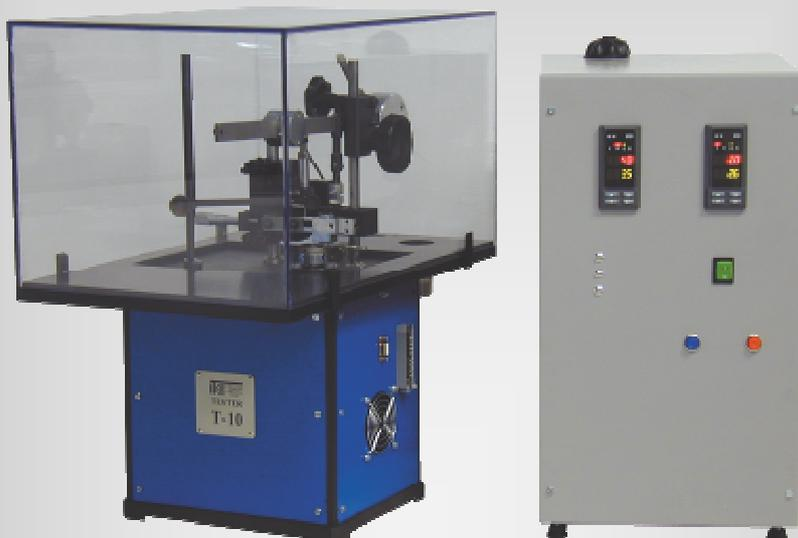
KS-10 chamber, made of a transparent material, is easily and quickly mounted onto T-10 Testing Machine and is equipped with a special air conditioner. The desired values of RH and temperature are set using the keys located on the front end of the air conditioner. The LED displays show the preset values as well as current values of RH and temperature inside the chamber.
