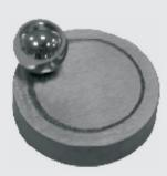
The tribosystem consists of the stationary ball pressed at the required load P against the disk rotating at the defined speed n. The disk is made of the tested material. When testing a surface coating, it is deposited on the disk. The friction couple is inserted in the insulated test chamber equipped with the heater H, which enables increasing the temperature and keeping it constant.
