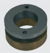
The tribosystem consists of the stationary ring pressed at the required load P against the disk rotating at the defined speed n. The friction couple is inserted in the insulated test chamber equipped with the heater H, which enables increasing the temperature and keeping it constant. It is possible to control the atmosphere by introducing a gas into the test chamber.
