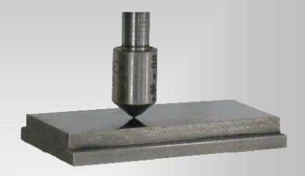
The tribosystem consists of the stationary indenter pressed at the required load P against the plate sliding at the defined velocity v. The plate is made of the tested material. In case of testing of a surface coating, it is deposited on the plate.
