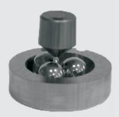
In case of testing of an effect of lubricants on pitting, the tribosystem consists of the three bottom balls (2), free to rotate in the special race (3) and pressed at the required load P against the top ball (1). The top ball is fixed in the ball chuck and rotates at the defined speed n.
