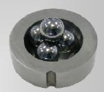
During testing of EP, AW properties, and friction coefficient the tribosystem (figure on the left) consists of the three stationary balls (2) fixed in the ball pot (4) and pressed at the required load P against the top ball (1). The top ball is fixed in the ball chuck (3) and rotates at the defined speed n. The ball pot (4) is equipped with a heater.
